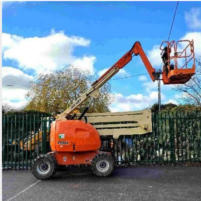
Example of an MEWP for use by trained operatives only.
